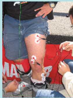
Fig. 2. EMG electrodes being applied to the skier's legs.
